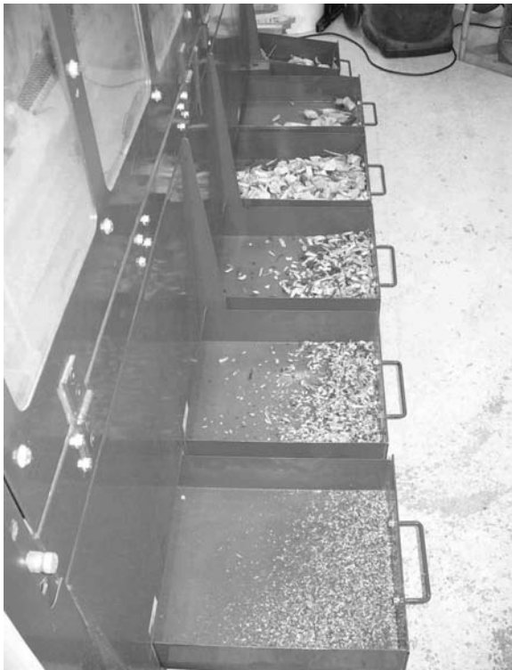
Figure 8.3: Separation of wood chip particles into size categories in the rotary sieve.
