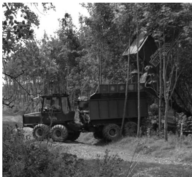
Figure 2.8: The Silvatec chip forwarder.
