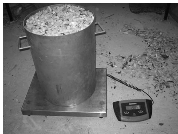
Figure 2.3: Stainless steel pot for the bulk density measurement.
