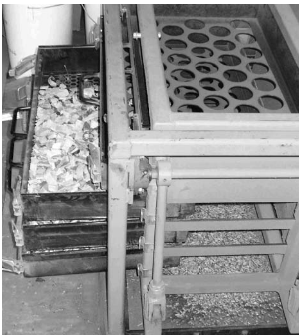
Figure 2.2: The oscillating screen for size distribution measurement of the chips.
