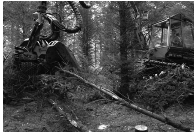
Figure 2.4: The Gremo harvester producing energy wood tree section.
