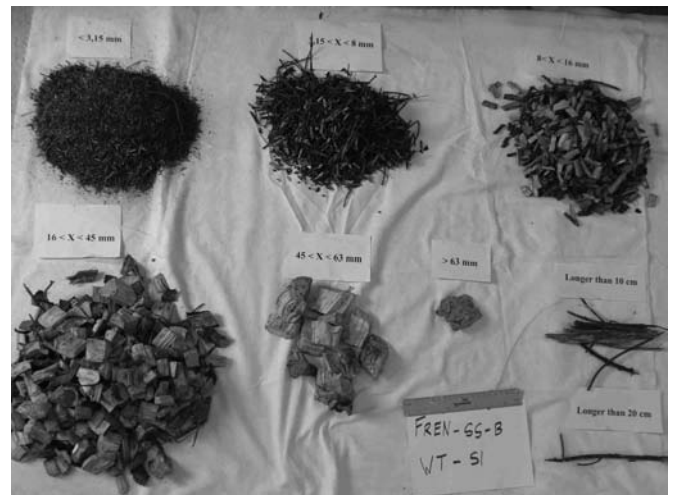
Figure 8.4: Wood chip assortment sub-sample divided into particle size categories.
